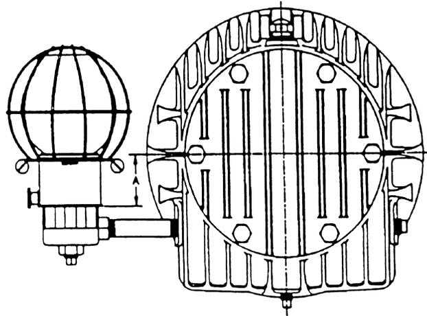
Whenever refilling system with oil, NEVER pour oil directly into oiler base. Always fill oiler bottle and invert onto oiler base. Never interchange micrometer leveling rods.
