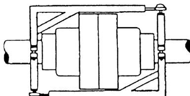
**Single dial indicator method** - used to measure parallel and angular misalignment. An alternative method is by use of a single dial indicator to measure both parallel and angular misalignment (see figures 10,11 & 12).
