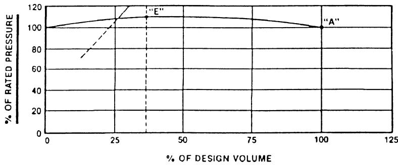
There is no such thing as a "surgeless" centrifugal. However certain impeller sizes and configurations may exhibit such light surge that no mechanical damage to the machine will occur.
